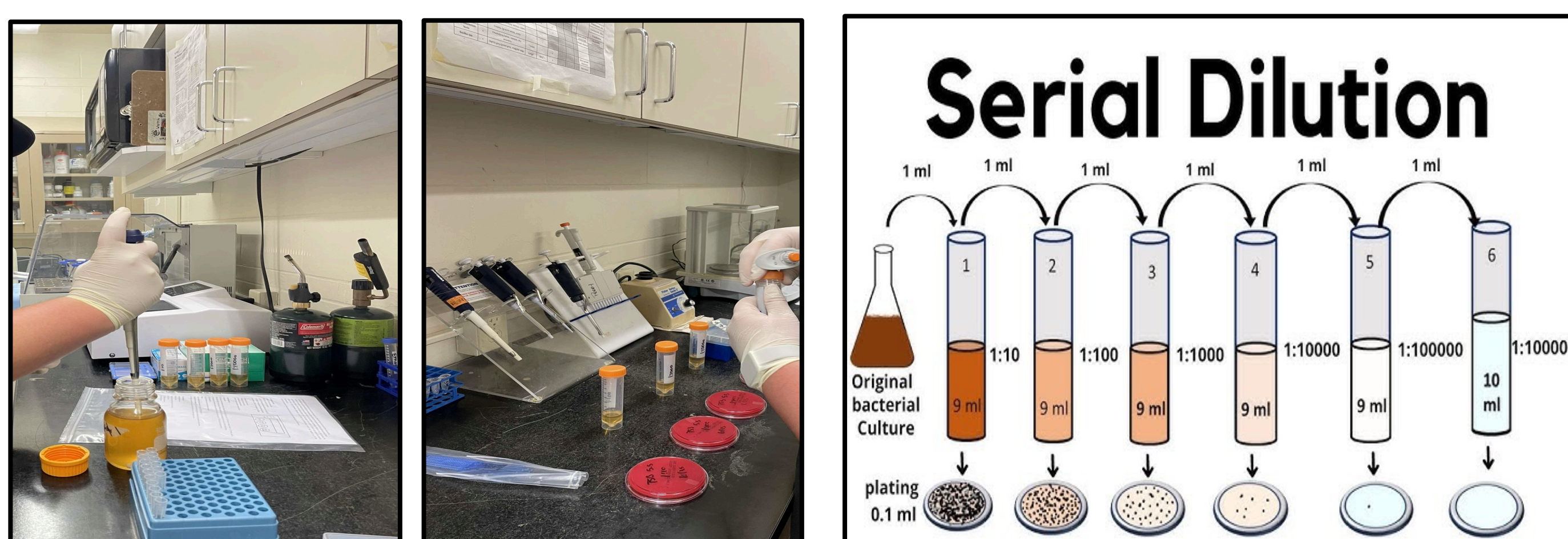
Figure 4: Representation depicting the formulation of the teat dip solution. Specifically, the broth bacterial concentration being checked by running the plate dilution series and spectrophotometer measurements.
